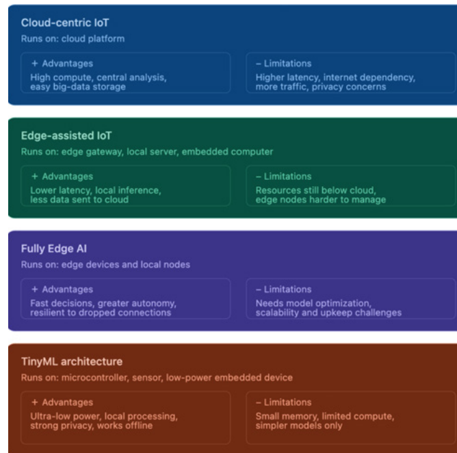
Figure 10. Comparative overview of cloud-centric IoT, edge-assisted IoT, fully Edge AI, and TinyML architectures, highlighting their execution environments, main advantages, and key limitations.
