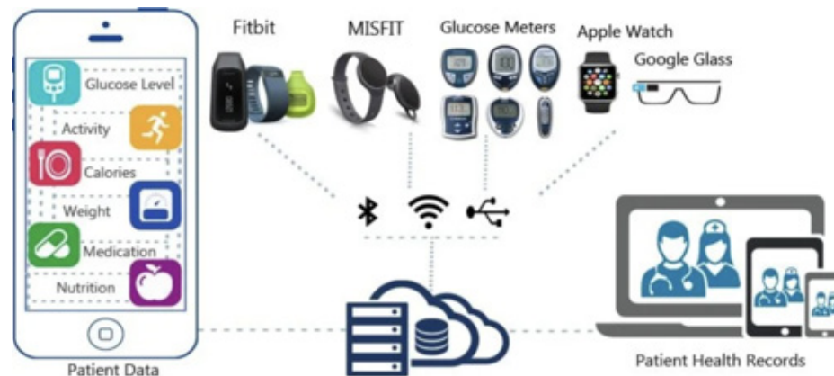
Figure 7. Wearable IoT-based healthcare system showing the connection between patient-generated data, wearable and medical monitoring devices, cloud infrastructure, and electronic patient health records.
