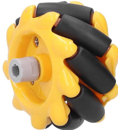
Figure 2: Mecanum wheel specific to the UNTLab platform
